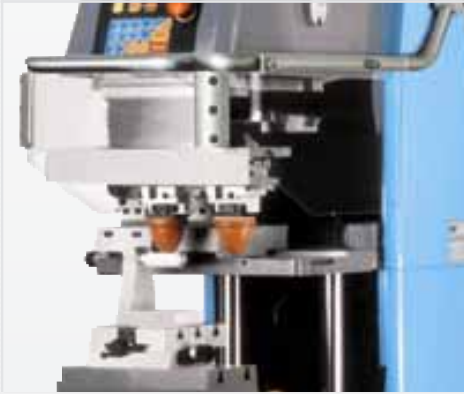
Reciprocatore tamponi SP 114 e tavola ortogonale TO 100 su Logica 100 Shuttle system SP 114 and cross table TO 100 fixed on Logica 100
