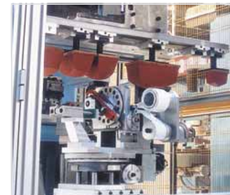
Dispositivo multiasse (TRCN 2.5 + TRCN 03) su indexore PRE 1370 Multi-axis device (TRCN 2.5 + TRCN 03) on indexor PRE 1370
