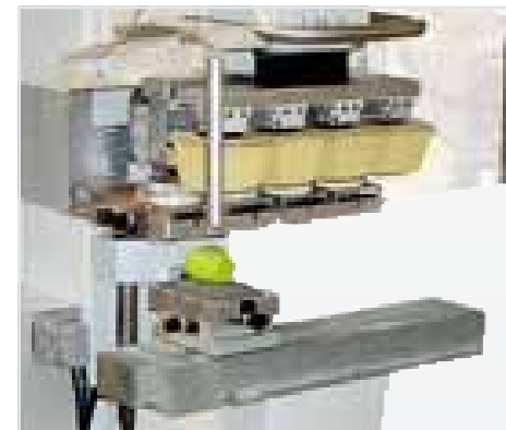
Indexore PL 450 e tavola ortogonale TO 100 su Logica Micro LP Indexer PL 450 and cross table TO 100 fixed on Logica Micro LP
